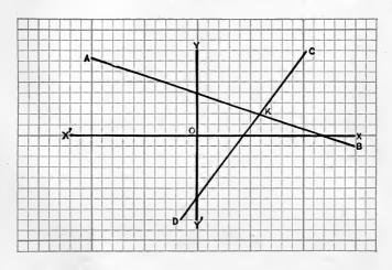
445. Graph of the Solution of a Pair of Simultaneous Linear Equations. In the figure the straight line AB is the graph of the equation x + 3y = 12, and the straight line CD is the graph of the equation 4x - 3y = 18. It is evident that the coördinates of K, the point of intersection of the lines AB and CD, must satisfy both equations.
