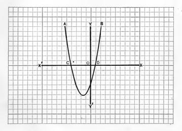
Plot the points found  $(-1.5, -6\frac{1}{4})$ , (-1, -6), (-2, -6), and so on. Through these points with a free hand draw the smooth curve AB. The curve AB is the graph of the function  $x^2 + 3x - 4$ . This graph consists of one symmetrical branch of infinite length and is called a parabola. For values of y less than  $-6\frac{1}{4}$ , the corresponding values of x are imaginary.
