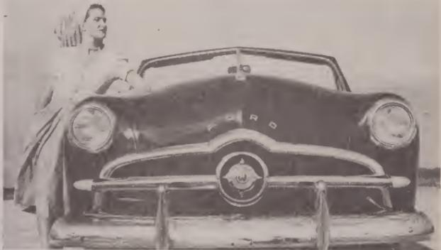
The smooth, flowing lines of the 1949 Ford passenger cars are accented by the simplicity of the air-scoop grille. Fresh air for the pressurized ventilation system also enters through the grille. The distinctive styling of the 1949 Ford convertible features smooth, flowing contours, full fender-width body and luxurious interior appointments. Completely new, the convertible chassis is doubly reinforced.
